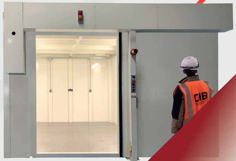
Large Cabinet with automatic sliding door 2.8x3.0x2.8m, 10mm lead, 17tons
